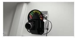
There are two different types of projectors used in multi-sensory rooms. Projectors which can be used with an iPad or computer which we will look at later in the module and wheel projectors like this.
